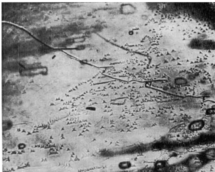
Figure 4. The effect of cleavage on the dislocation content of benzoic acid crystals-water etch ( 100\times ) (cf. Fig. 1).
